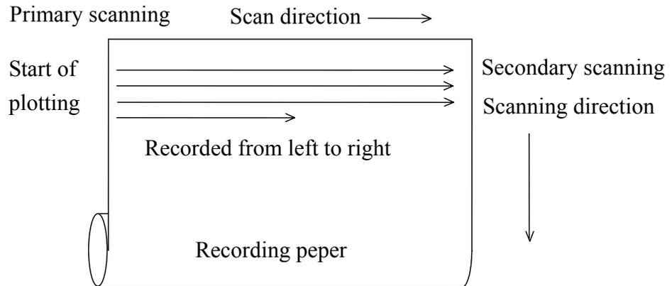
**Primary scanning** Scanning in the horizontal direction as shown above
