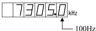
For example, the frequency 7305 kHz for JMH can be preset in the following procedure.
