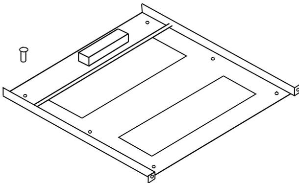
Fix the mounting base on a desk or stand, using wooden screws or M6 screws.
