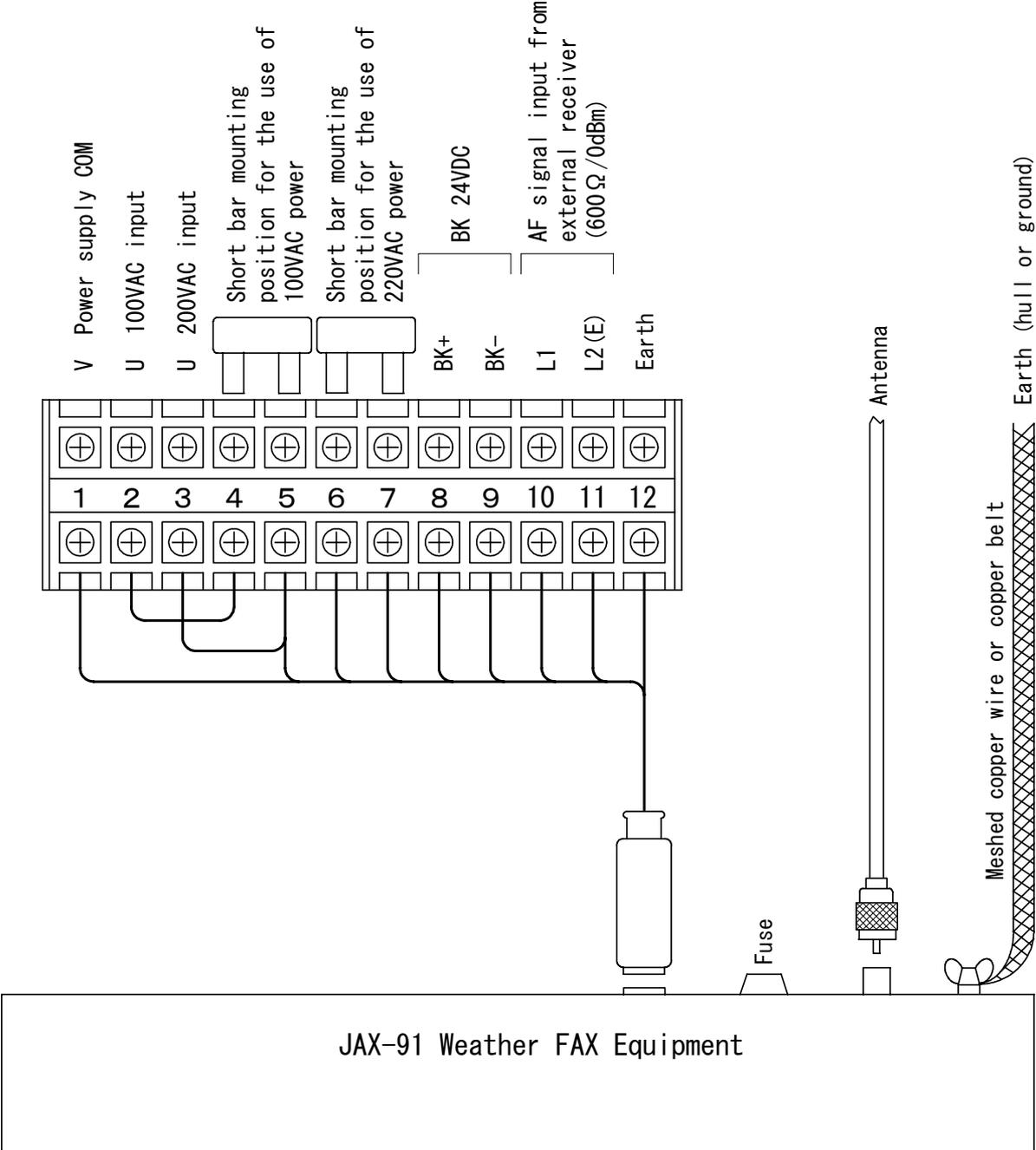
JAX-91 Weather FAX to External Terminals Connection Diagram
